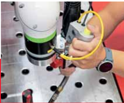
Simple welding path programming with direct torch guidance
