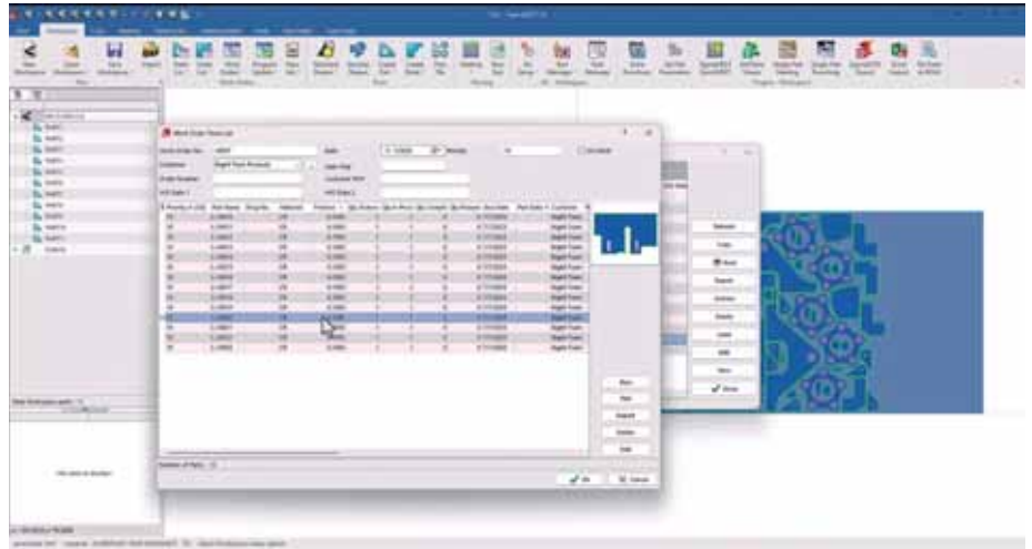
SigmaNEST Task List gives users access to create and load jobs and apply commands to multiple jobs.
