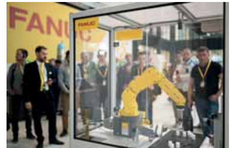
The FANUC Education cell, controlled by a proprietary FANUC CNC unit, features all the real-world functions required to teach core robotics programming and operating skills and help inspire the next generation to realise their career ambitions
